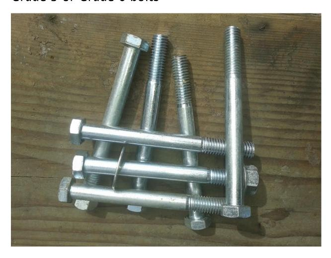
Holes drilled will align through three or more laminated 1½" lumber for upright posts to a span of 4½" thus requiring at least a 5" bolt when used with two washers, or 5½" bolt when utilizing a full sized locking nut for bolting the main sub-assemblies.
